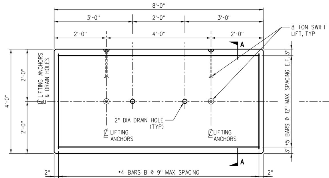
**4' x 8' PRECAST CONCRETE WINGWALL PANEL**
