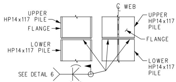
**ALTERNATE PILE SPLICE DETAIL 3**
