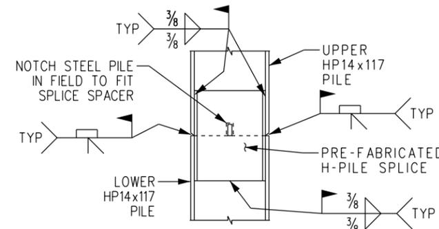
**TYPICAL PILE SPLICE DETAIL 5**
