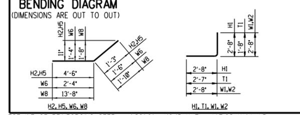
EST. WT. OF REINFORCING STEEL = 1,861.91 \* (10.15 X Z) + (47.98 X N) LB.
