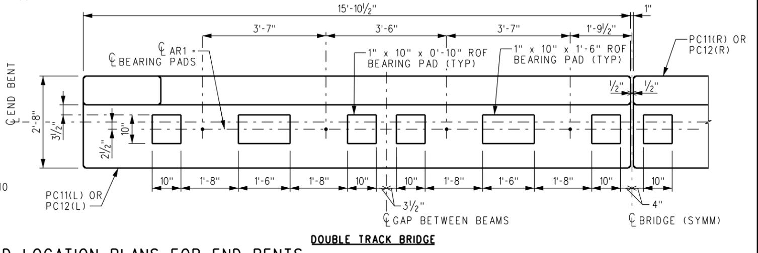
**ANCHOR ROD AND BEARING PAD LOCATION PLANS FOR END BENTS**
