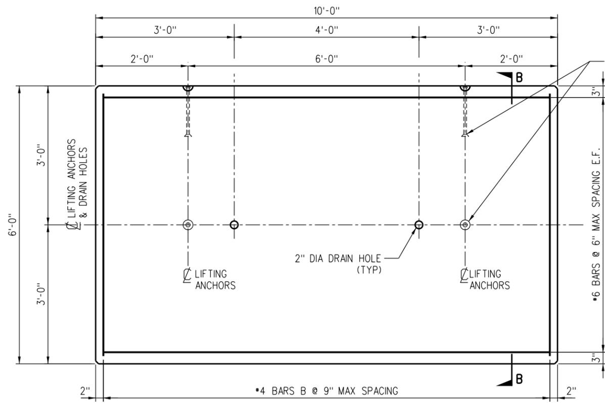
**6' x 10' PRECAST CONCRETE WINGWALL PANEL**
