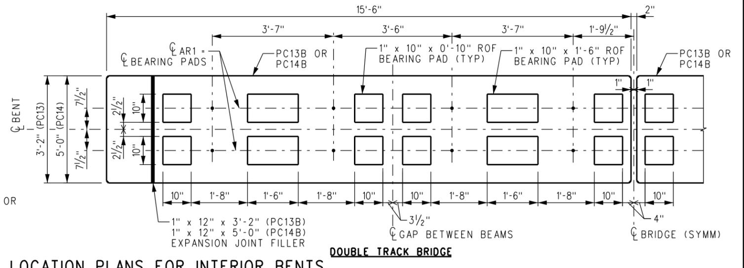
**ANCHOR ROD AND BEARING PAD LOCATION PLANS FOR INTERIOR BENTS**
