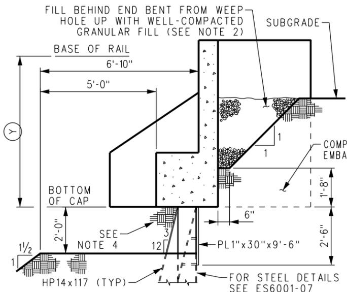
**ALTERNATE GRADING DETAIL 7**
