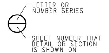
**SHEET SHOWING SECTION OR DETAIL CUT**
