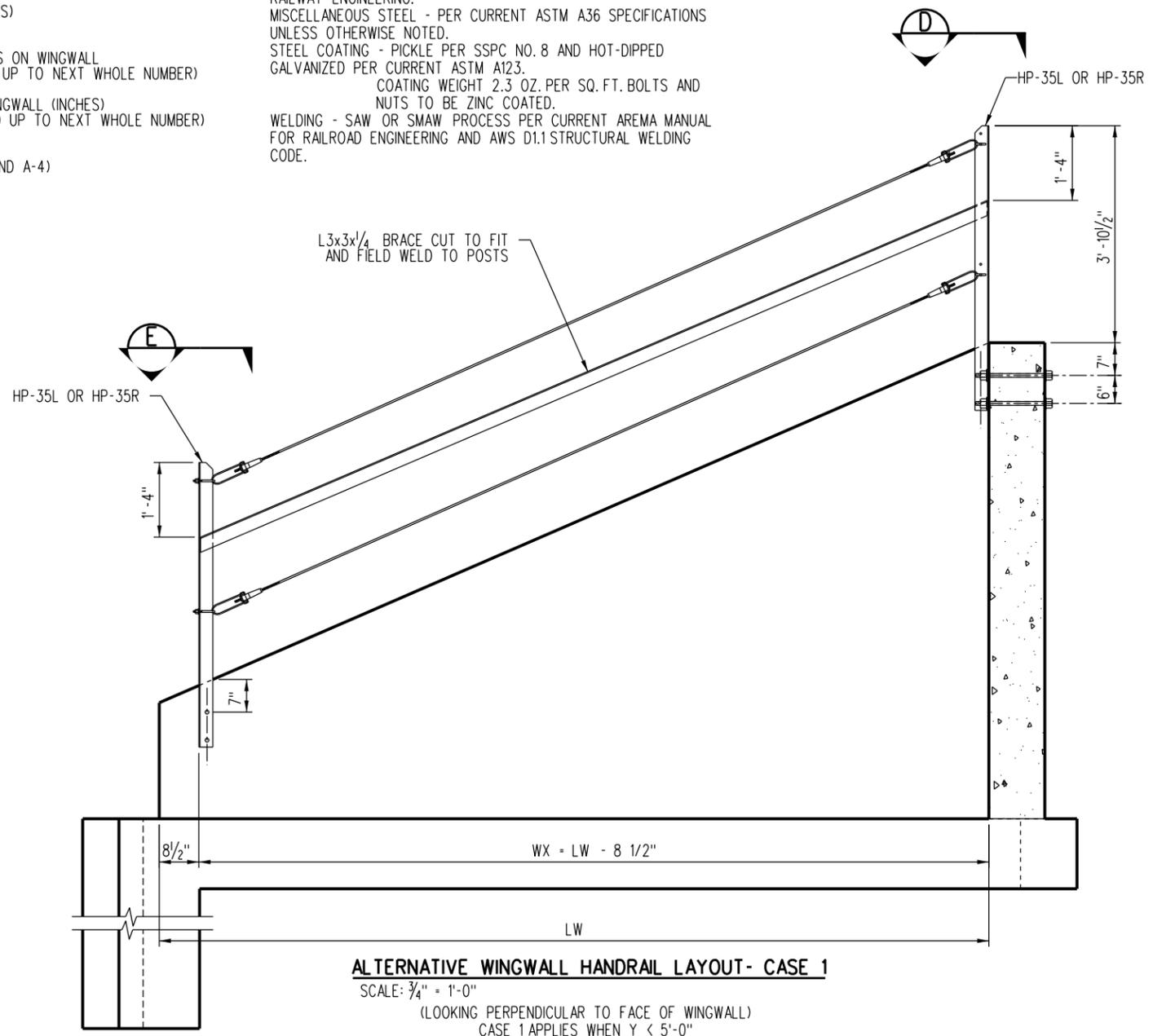
**ALTERNATIVE WINGWALL HANDRAIL LAYOUT- CASE 1**
