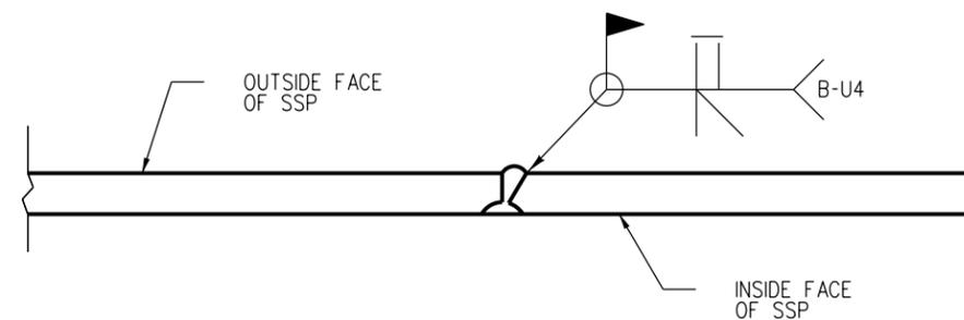
PIPE END WELD DETAIL
