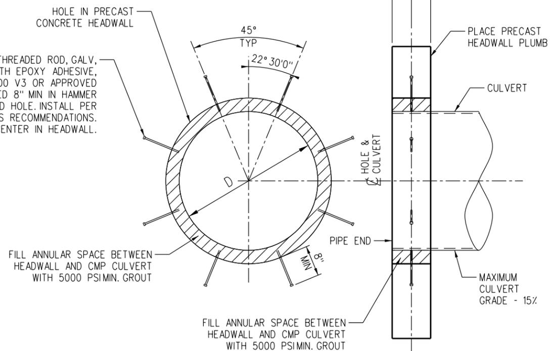
END ANCHOR INSTALLATION DETAIL
