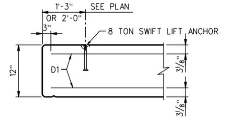
**LIFTING ANCHOR DETAIL**
