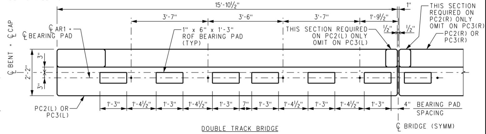
**ANCHOR ROD AND BEARING PAD LOCATION PLANS FOR END BENTS**
