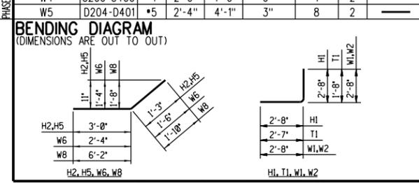
EST. WT. OF REINFORCING STEEL = 755.26 \* (6.50 X Z) + (35.46 X N) LB.
