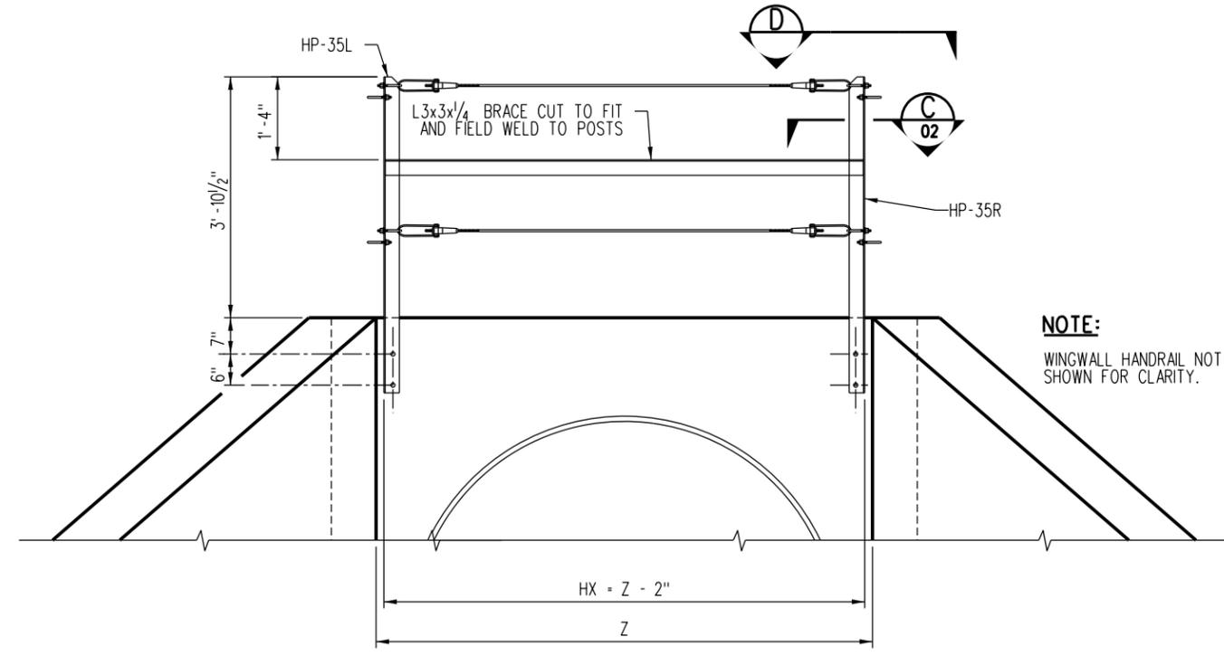
**ALTERNATIVE HEADWALL HANDRAIL LAYOUT-CASE 1**
