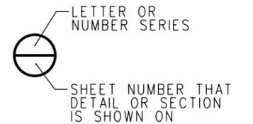
**SHEET SHOWING SECTION OR DETAIL CUT**
