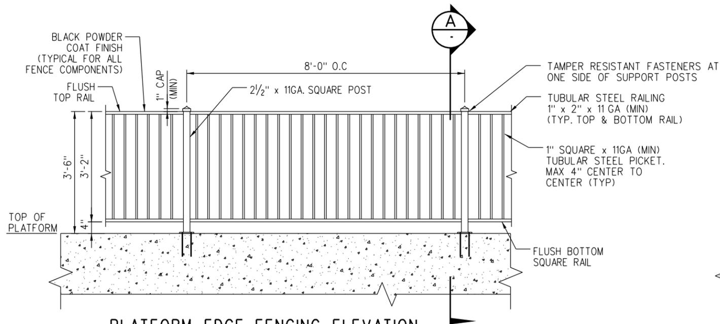
**PLATFORM EDGE FENCING ELEVATION**
