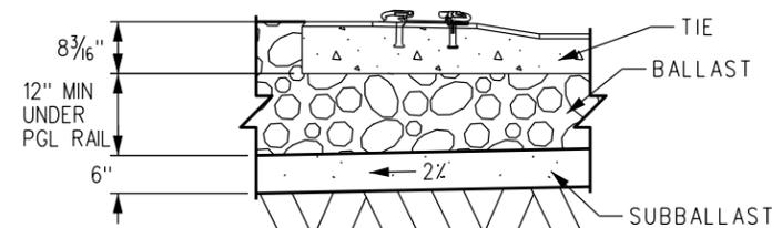
**ROADBED SECTION DETAIL FOR MAINLINE, SIDING TRACKS, & YARD TRACKS**
