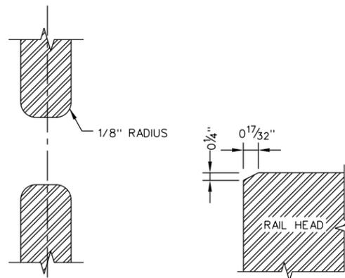
**BOLT HOLE CHAMFER SECTION A-A**
