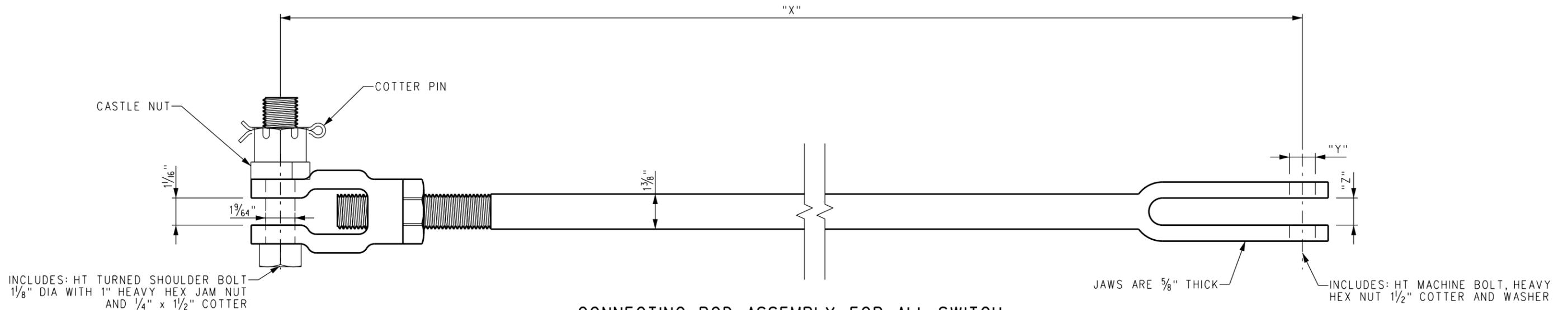
**CONNECTING ROD ASSEMBLY FOR ALL SWITCH STANDS WITH ADJUSTABLE CRANK EYE (22E, 36E-EH, 112E, ETC)**
