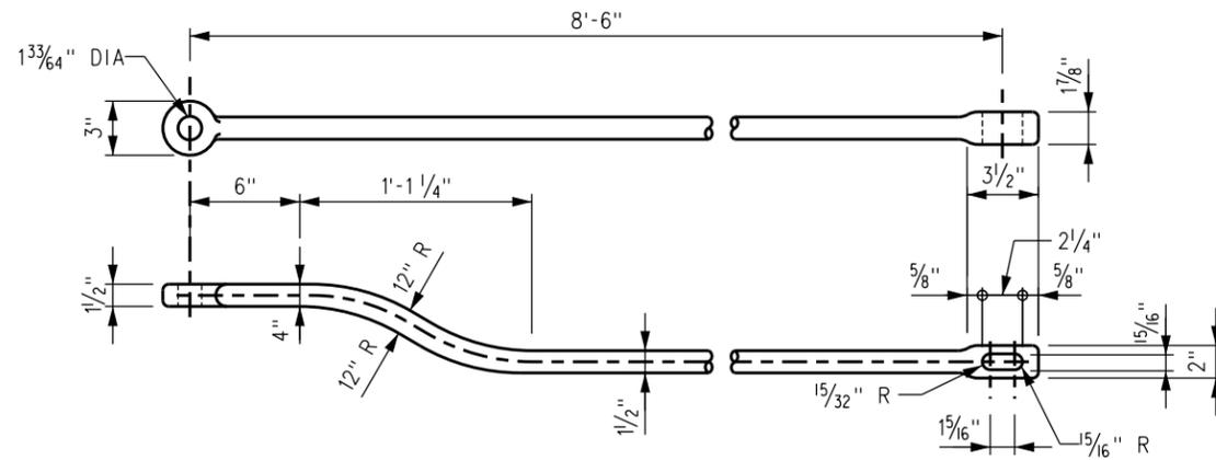
**CONNECTING ROD FOR USE WITH HAYES DERAIL AND HIGH OR LOW SWITCH STANDS PER SCRRA ES2701 & ES2704**
