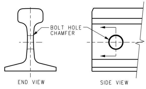
BOLT HOLE CHAMFERING
