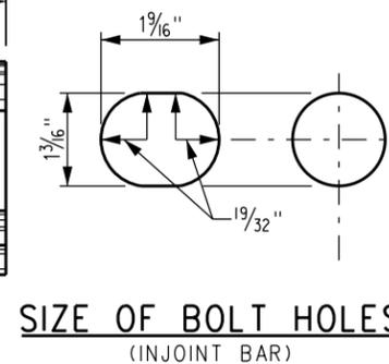
**SIZE OF BOLT HOLES (IN JOINT BAR)**
