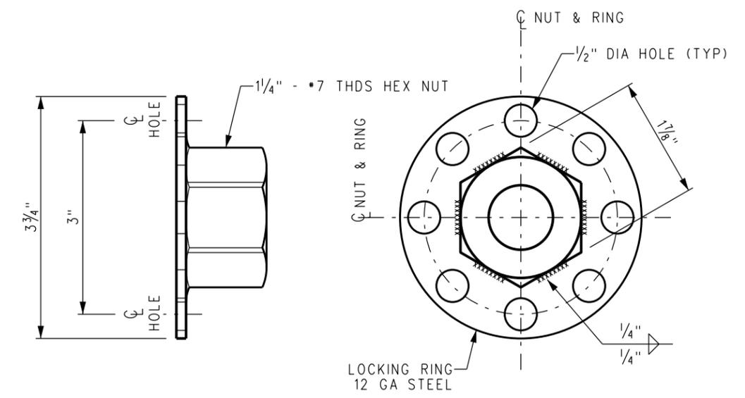
**DETAIL A - NUT AND LOCKING RING**
