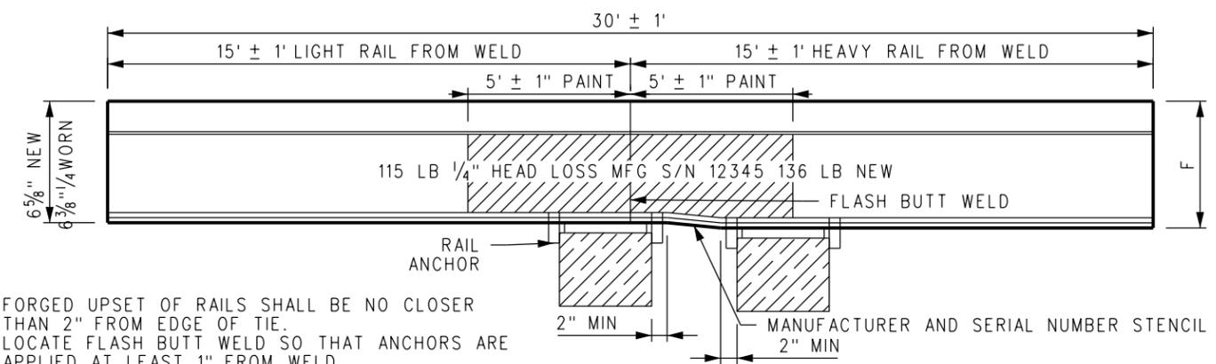
FORGED UPSET OF RAILS SHALL BE NO CLOSER THAN 2" FROM EDGE OF TIE. LOCATE FLASH BUTT WELD SO THAT ANCHORS ARE APPLIED AT LEAST 1" FROM WELD.
