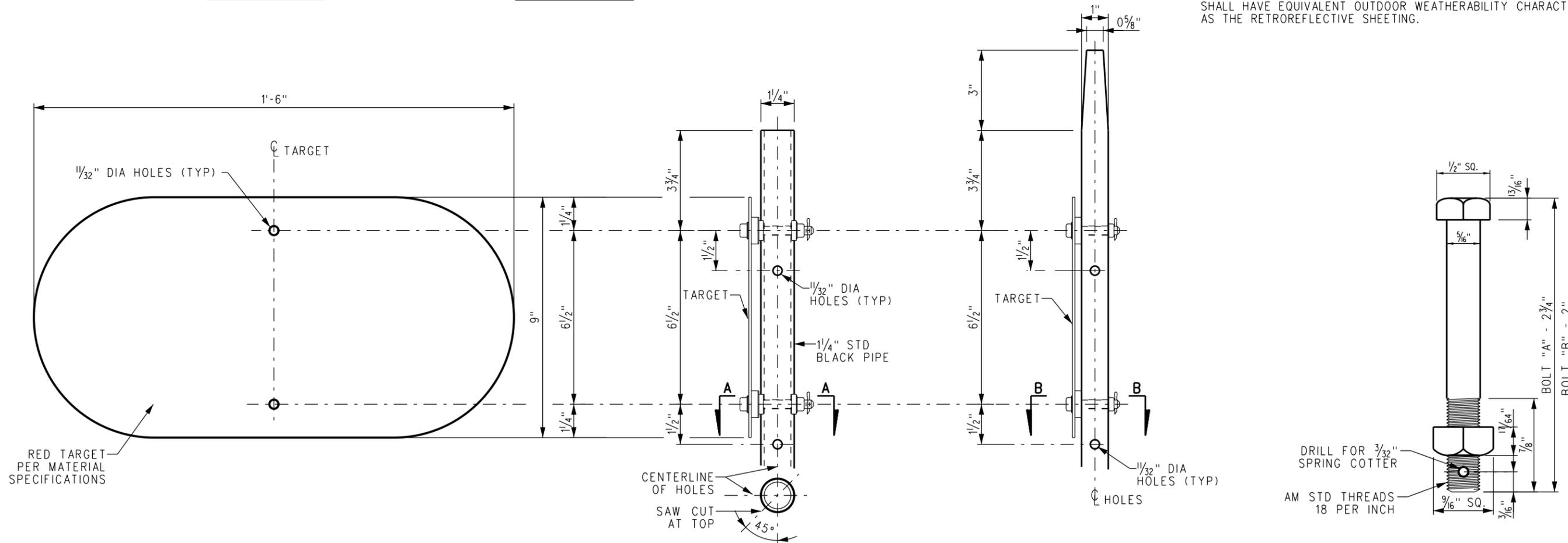
DERAILING SWITCH TARGET
