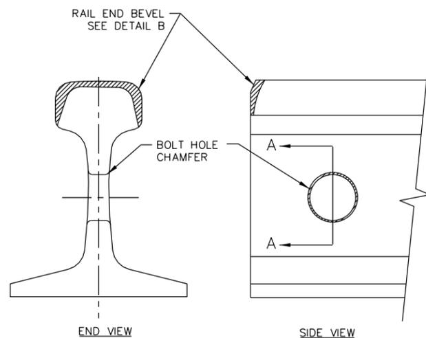
**RAIL CHAMFERING AND BEVELING**
