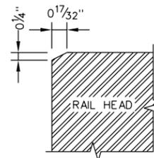
**RAIL END BEVEL DETAIL B**
