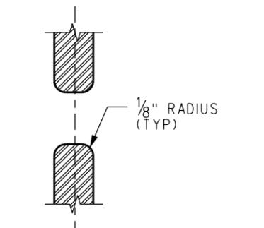
BOLT HOLE CHAMFER SECTION A-A
