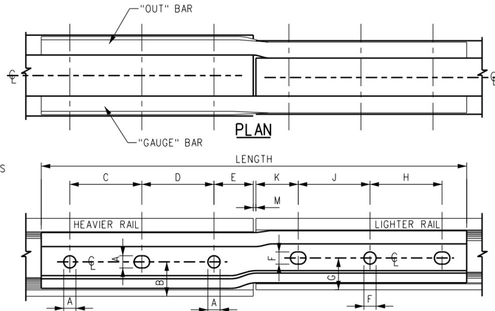
**ELEVATION OF "GAUGE" BAR**
