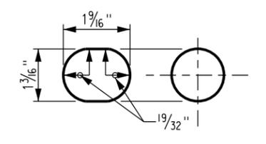
SIZE OF BOLT HOLES (IN JOINT BAR)
