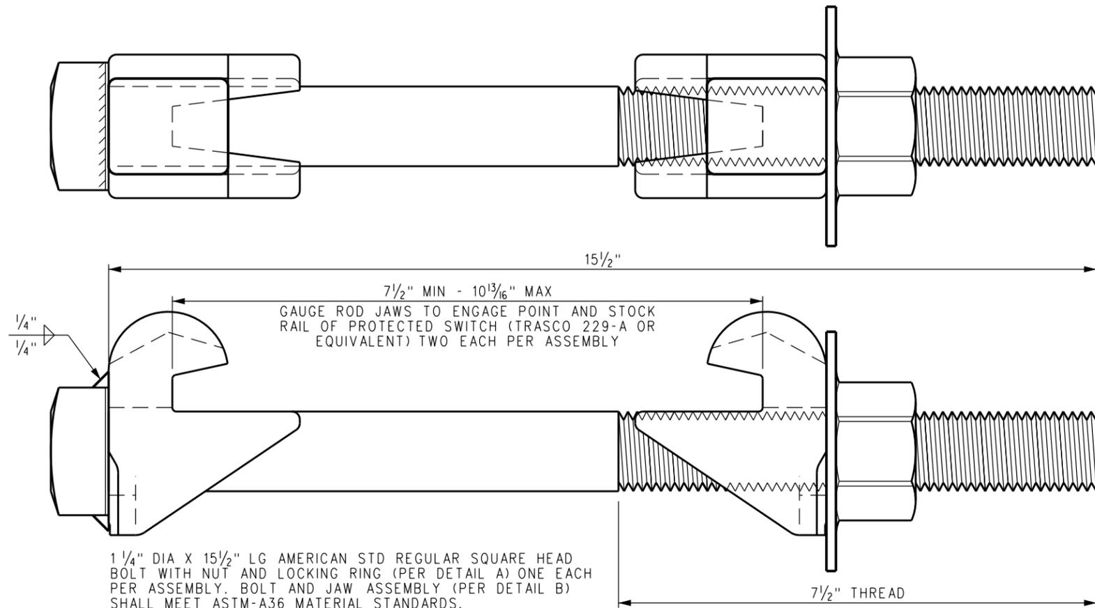
1 1/4" DIA X 15 1/2" LG AMERICAN STD REGULAR SQUARE HEAD BOLT WITH NUT AND LOCKING RING (PER DETAIL A) ONE EACH PER ASSEMBLY. BOLT AND JAW ASSEMBLY (PER DETAIL B) SHALL MEET ASTM-A36 MATERIAL STANDARDS.
